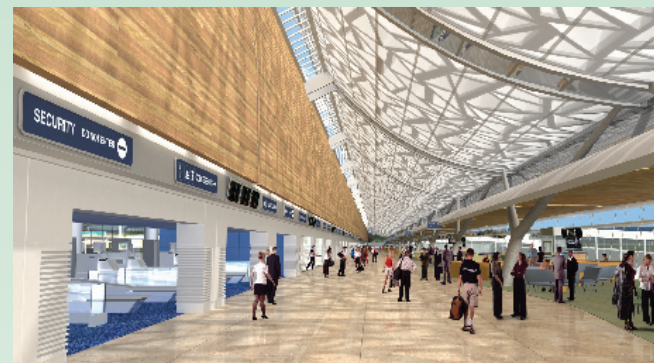
The trelliswork roof at San Jose International's North Concourse will act similar to a skylight and allow natural light into the area.
